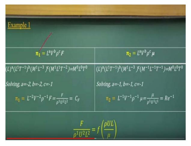
Now to look at that this is a called a  $\pi$  —theorem it is a very easy concept that though please do not have a conclusion with the  $\pi$  means 3.14 it is a non dimensionless form of p is okay. So if it is that I can have a 3 variables okay that is the length velocity and the  $\pi$  and the force these are called the repeating variables length velocity and viscosity I will put the repeating variables and with the F.
