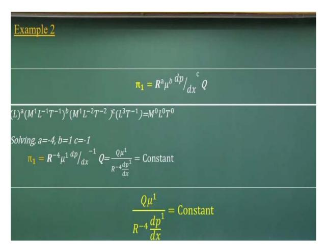
We will follow the same concept I am not going to repeat it here again you put a substitutes of power x point of abc substitute this dimensional values and equate with non-dimensional value you will get abc value and finally we will get a the relationship between the 4 which will make a non-dimensional group it is a very example simple things but first thing is that we should remember the dimensions of the fluid variables.
