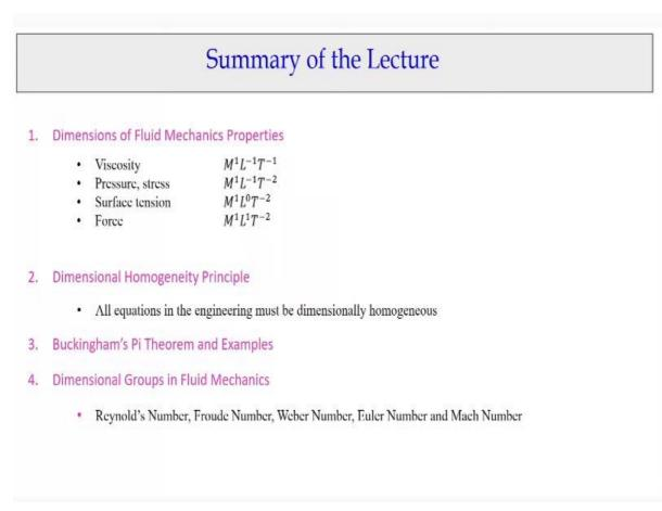
Viscosity  $M^1L^{-1}T^{-1}$  Pressure, stress  $M^1L^{-1}T^{-2}$  Surface tension  $M^1L^0T^{-2}$  Force  $M^1L^1T^{-2}$
